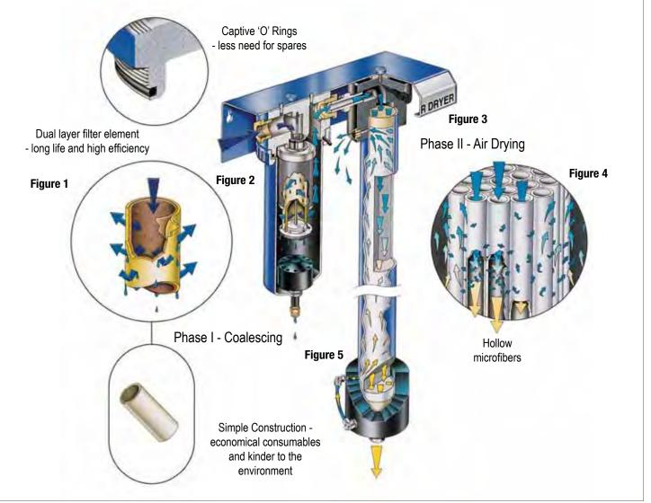
Membrane Air Dryer - Principal of Operation
